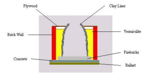
The tandoor is surrounded by vermiculite insulation, to a minimum thickness of 100mm. This reduces the rate at which heat is lost from the tandoor, reducing the fuel consumption. The insulation is retained by brick walls which also support the working surface on the top of the structure. The working surface is exterior-grade plywood with a hole through which the mouth of the tandoor protrudes.
